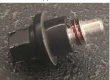
5. Assemble the knob with the sleeve to each of the links. Apply pressure while turning the knob so that the sleeve enters the slot of the end frame.
