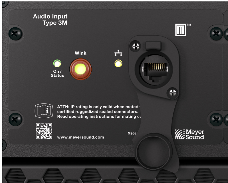
Type 3M Milan Endpoint Module, On/Status LED, Wink Button/LED, Network Connection LED, and Network Connector
