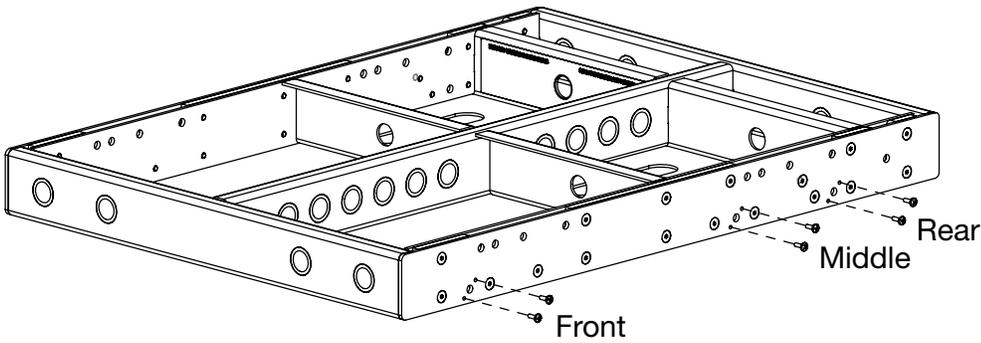
Blanking Screws (6 per side) to Prevent Corrosion at Unused Pin Locations for Ultra Weather Protection Grid
