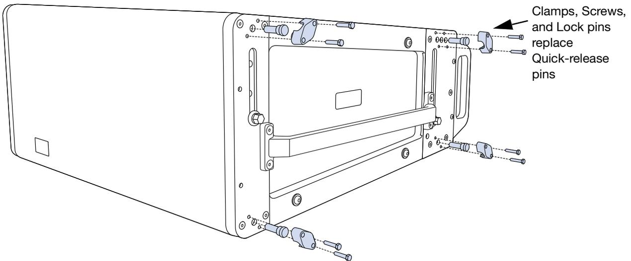
Ultra Weather Protection LEOPARD Loudspeaker Version has Clamps, Screws, and Lock pins that replace standard version quick-release pins
