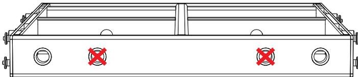
*Laser or Inclinometer Aiming Holes not Pickup Points*
