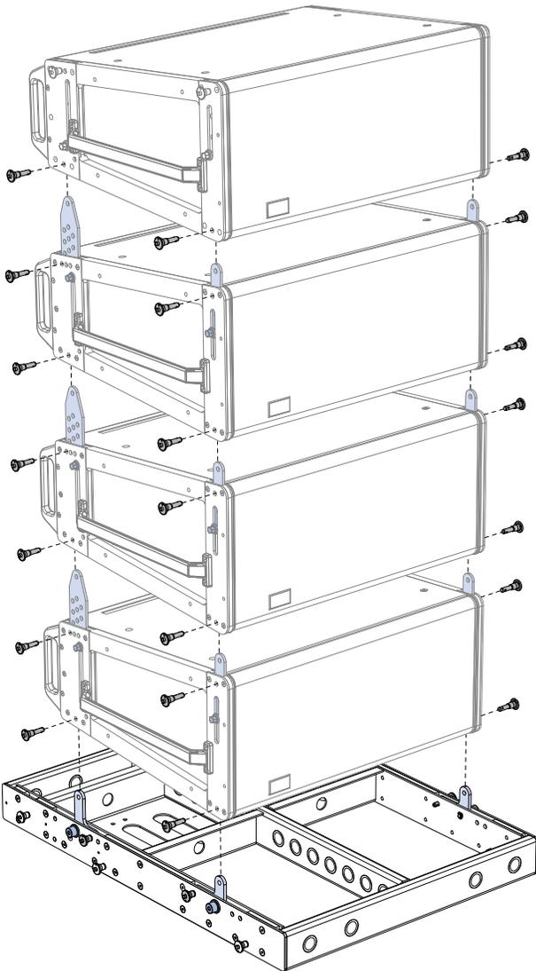
*MG-LEOPARD/900-LFC Grid with Groundstacked LEOPARDs, Exploded View*
