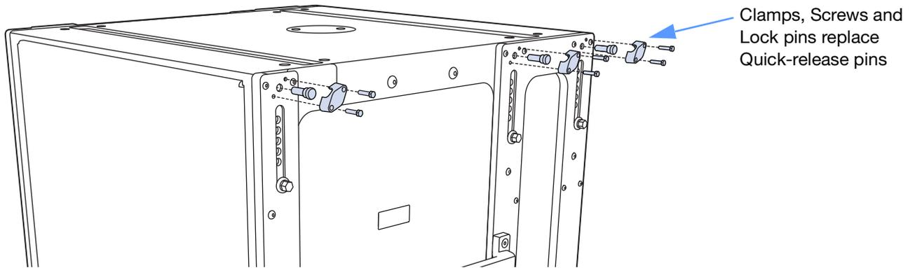
*Ultra Weather Protection 900-LFC Loudspeaker Version has Clamps, Screws, and Lock pins that replace standard version quick-release pins*
