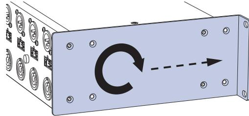
3. Use a #2 Phillips screwdriver to re-install the screws to secure the rackmount brackets to the enclosure.
