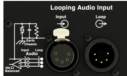
Figure 10: XLR 5-Pin Audio Connectors, Input and Loop Output
